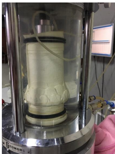
Figure 47 Treated 16 -0.50CaCl 2 -100, deformed shape (during and post-failure) and collected specimen
