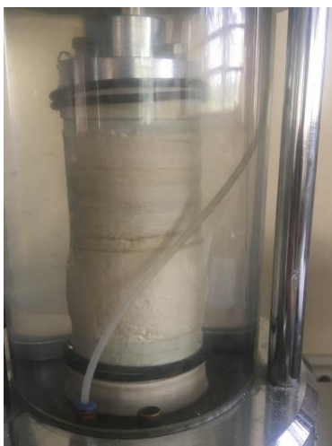
Figure 42 Treated_16_0.25CaCl2_200, deformed shape (during and post-failure) and collected specimen
