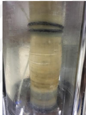
Figure 36 8 injections - 0.50 M \text{CaCl}_2 case control tests (a) after completing injections (b) while transferring the oven (c) after oven dried (d) while transferring the pedestal
