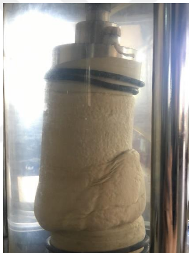
Figure 37 Deformed shape of untreated sand (Left is during the test, right is the post-failure shape) (a) 100 kPa (b) 200 kPa (c) 400 kPa
