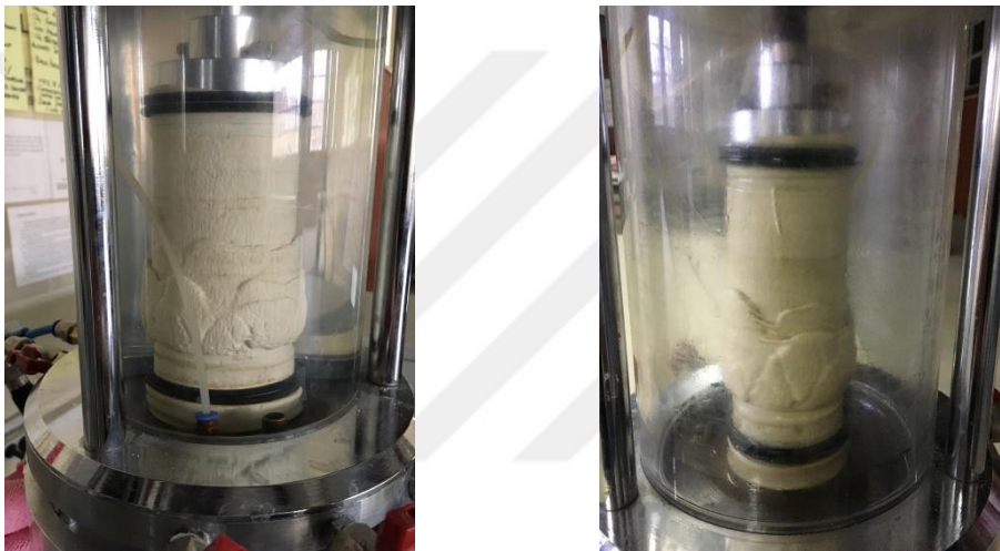
Figure 48 Treated_16_0.50CaCl2_200, deformed shape (during and post-failure) and collected specimen
