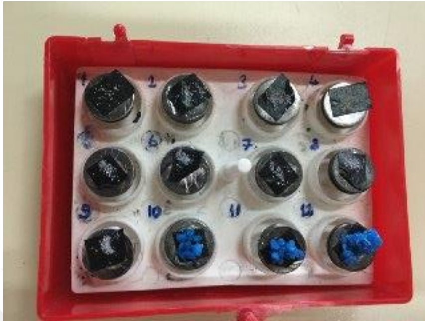
Figure 54 SEM samples placed on the conductive adhesive tab
