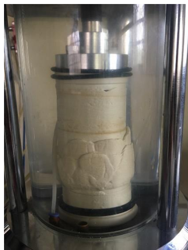
Figure 44 Treated_08_0.50CaCl2_100, deformed shape (during and post-failure) and collected specimen (specimen couldn't be collected at two pieces)
