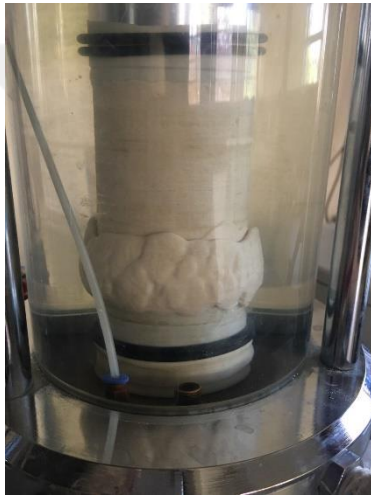
Figure 40 Treated_08_0.25CaCl 2 _400, deformed shape (during and post-failure) and collected specimen
