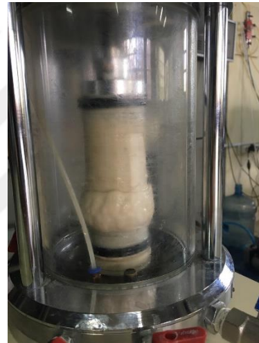
Figure 40 Treated_08_0.25CaCl 2 _400, deformed shape (during and post-failure) and collected specimen
