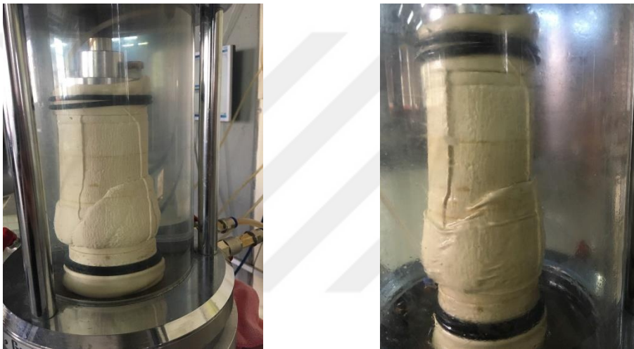
Figure 45 Treated_08_0.50CaCl2_200, deformed shape (during and post-failure) and collected specimen
