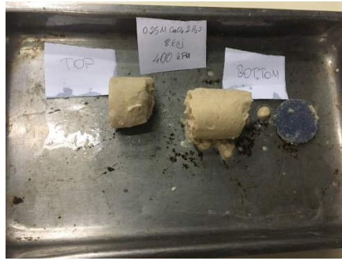
Figure 40 Treated_08_0.25CaCl 2 _400, deformed shape (during and post-failure) and collected specimen
