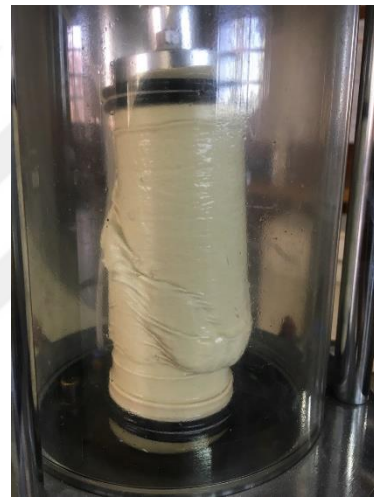
Figure 44 Treated_08_0.50CaCl2_100, deformed shape (during and post-failure) and collected specimen (specimen couldn't be collected at two pieces)
