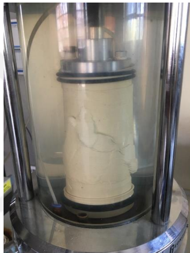
Figure 44 Treated_08_0.50CaCl2_100, deformed shape (during and post-failure) and collected specimen (specimen couldn't be collected at two pieces)
