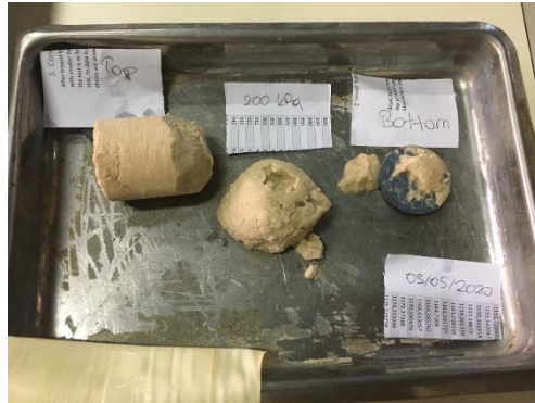
Figure 45 Treated_08_0.50CaCl2_200, deformed shape (during and post-failure) and collected specimen
