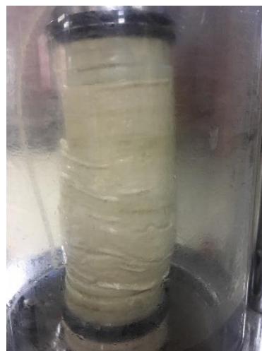
Figure 39 Treated_08_0.25CaCl2_200, deformed shape (during and post-failure) and collected specimen
