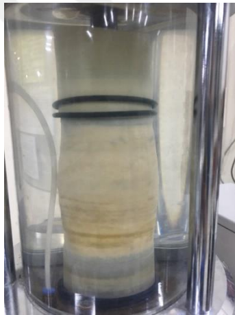
Figure 36 8 injections - 0.50 M \text{CaCl}_2 case control tests (a) after completing injections (b) while transferring the oven (c) after oven dried (d) while transferring the pedestal
