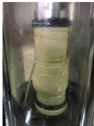
Figure 44 Treated_08_0.50CaCl2_100, deformed shape (during and post-failure) and collected specimen (specimen couldn't be collected at two pieces)
