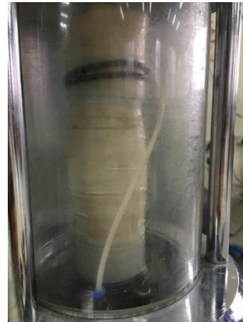
Figure 37 Deformed shape of untreated sand (Left is during the test, right is the post-failure shape) (a) 100 kPa (b) 200 kPa (c) 400 kPa
