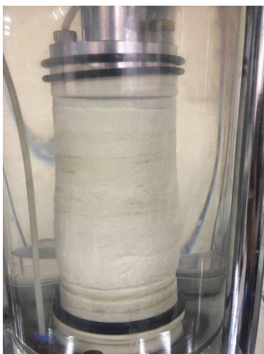
Figure 39 Treated_08_0.25CaCl2_200, deformed shape (during and post-failure) and collected specimen
