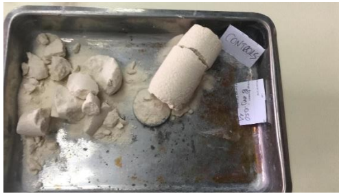
Figure 36 8 injections - 0.50 M \text{CaCl}_2 case control tests (a) after completing injections (b) while transferring the oven (c) after oven dried (d) while transferring the pedestal
