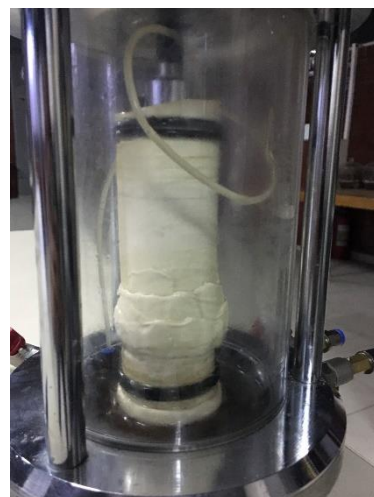
Figure 47 Treated 16 -0.50CaCl 2 -100, deformed shape (during and post-failure) and collected specimen
