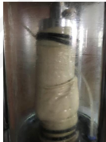
Figure 37 Deformed shape of untreated sand (Left is during the test, right is the post-failure shape) (a) 100 kPa (b) 200 kPa (c) 400 kPa
