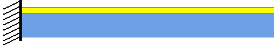
Figure 2.5 Schematic depiction of accumulation of a Au layer on top of a monolayer uniform Ni microcantilever
