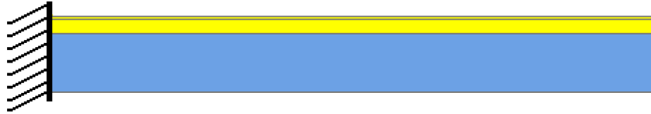
Figure 2.6 Schematic depiction of the 1 st incremental addition of Au layer on top of the initial bilayer uniform Ni-Au microcantilever
