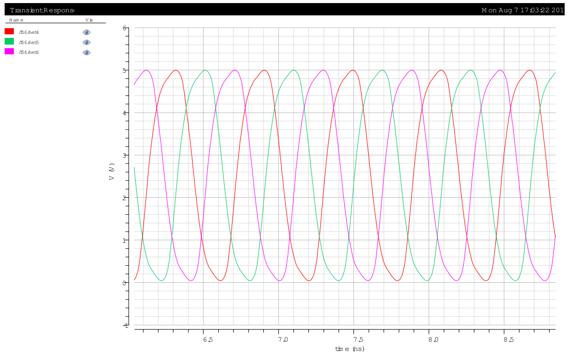
Figure 4.7: Oscillating signal at each stage of the three stage ring oscillator
