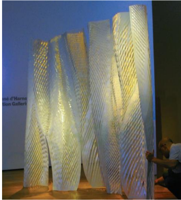
Figure 4.15: Laser cut and Folded geometry of Vector Wall (32) (Dunn, 2012: 142)
