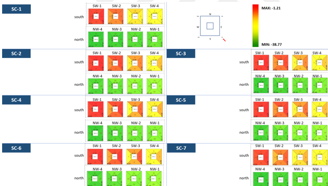
Figure D. 8 Façade Pressures for Wind Direction 135°
