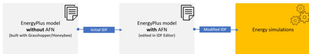
Figure 5.8. AFN integration into the energy model
