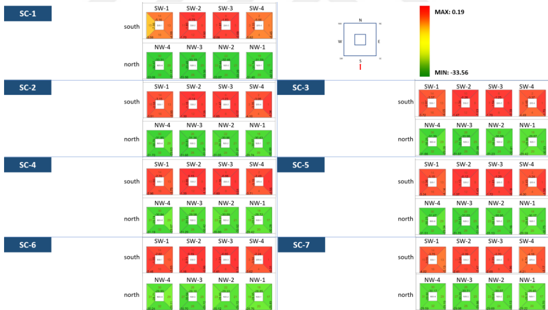
Figure D. 10 Façade Pressures for Wind Direction 180°
