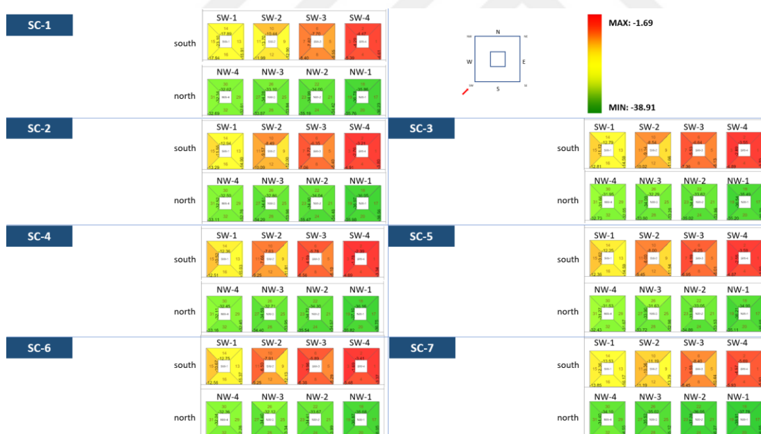
Figure D. 12 Façade Pressures for Wind Direction 215°
