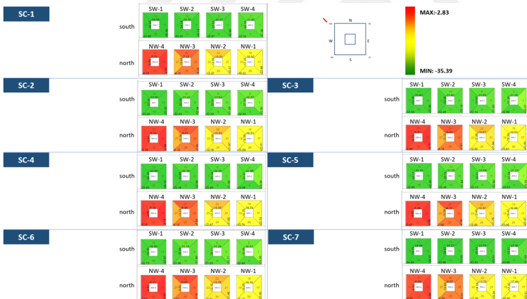
Figure D. 16 Façade Pressures for Wind Direction 315°
