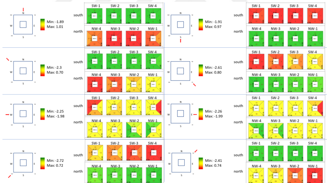
Figure C. 26 Façade Pressures for SC7
