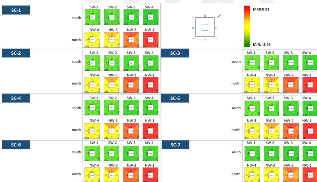
Figure D. 4 Façade Pressures for Wind Direction 45°
