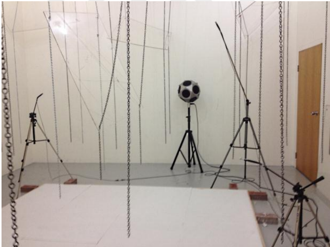
Figure 2.4: A photography showing reverberation room measurement set-up [4].
