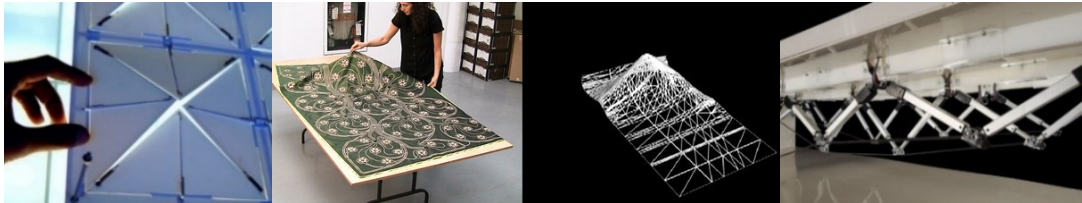
Figure 4.17. PixelSkin02 project, nickel-titanium alloys on façade as dynamic shape memory actuators (Above Left); IMBlanky project (Above Right); Variable Geometry Truss (Below)
