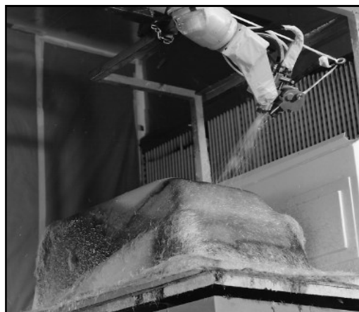
Figure 1.6 Spray-up process (Mazumdar, 2002)
