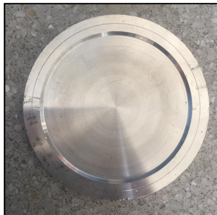
Figure 3.3 Mold 3, circular aluminum mold (Personal archive, 2018)
