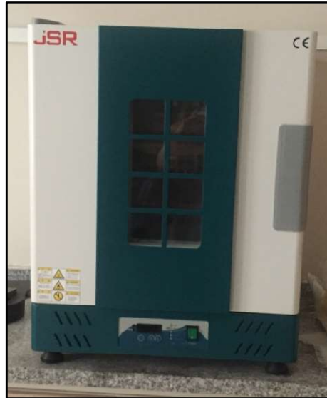
Figure 3.9 JSR brand JSOF-050 forced convection oven (Personal archive, 2018)
