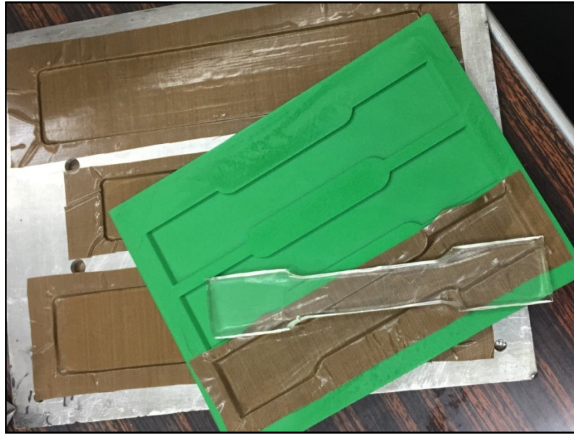
Figure 3.4 Coated molds with the self-adhesive teflon fabric (Personal archive, 2018)
