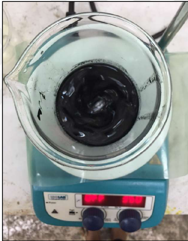
Figure 3.8 Magnetic stirrer machine and mixing epoxy resin and mineral (Personal archive, 2018)
