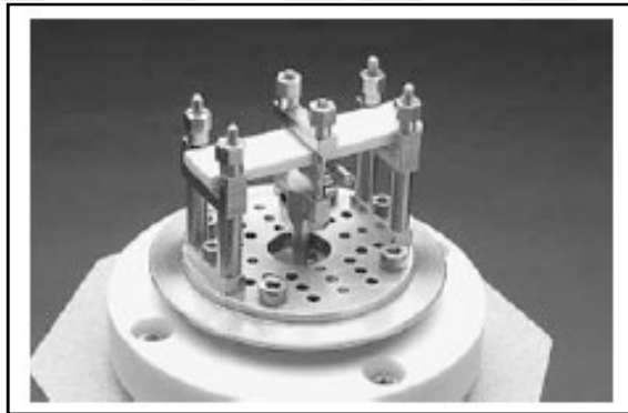
Figure 6.3 Three point bending test apparatus – dual cantilever (Menard, 2008)
