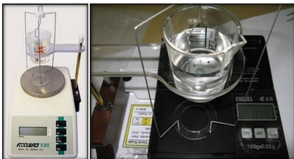
Figure 3.7 Gemmological specific gravity apparatus for sensitive measurement of the weight in air and the weight in water of Oltu-stone.
