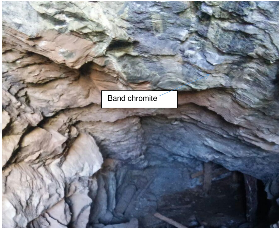
Figure 4.9. Band chromite surrounded by a dunitic envelope at the entrance of the underground mine
