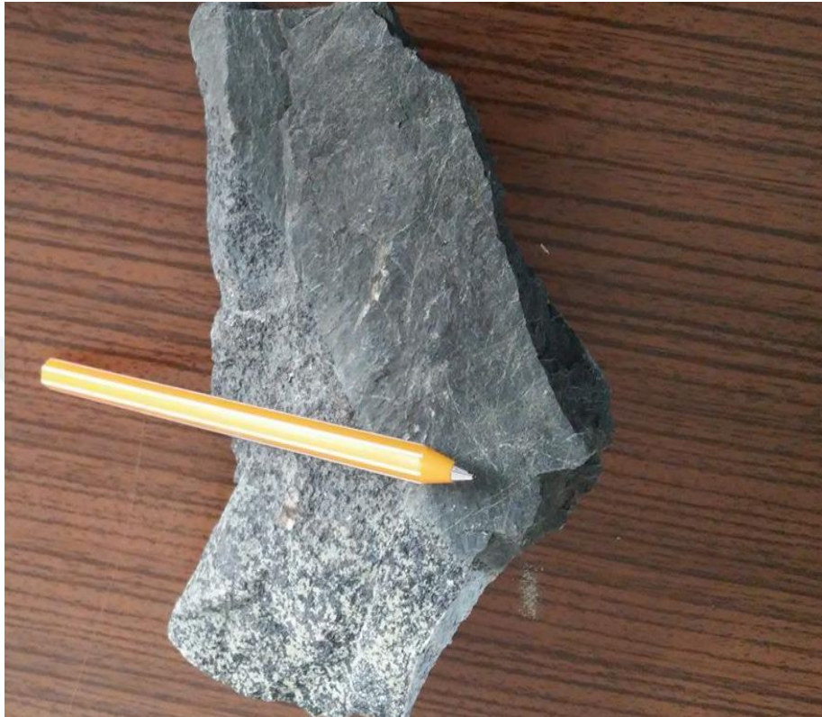
Figure 4.12. Harzburgite and disperse chromite ore boundary
