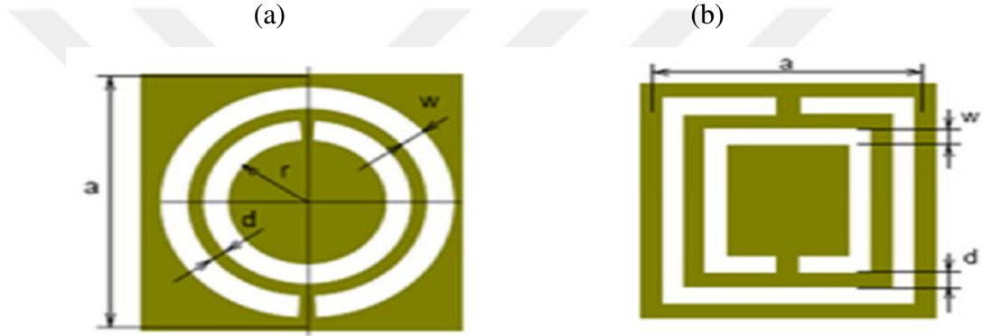
Figure 1.3 Complementary SRR structures: a) circular, b) rectangular [22]
