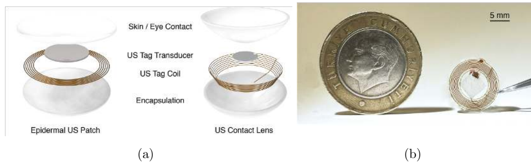
Figure 4.4: Concept of the US tags: (a) Exploded view of the epidermal US patch and US contact lens. (b) Photograph of a US tag next to a 1 Turkish Lira coin for scale.
