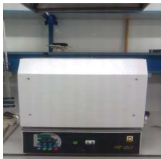
Figure 3.5 Drying oven for operation at 103-105 °C Figure 3.6 Muffle furnace for operation 550 °C
