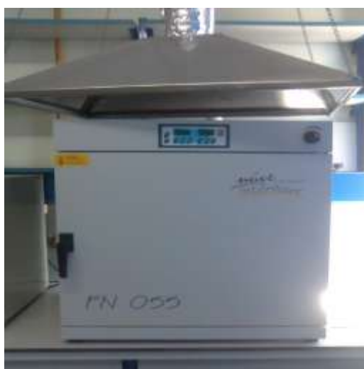
Figure 3.5 Drying oven for operation at 103-105 °C Figure 3.6 Muffle furnace for operation 550 °C
