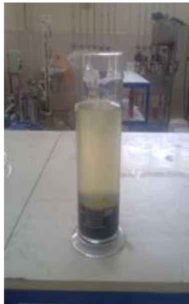
Figure 3.8 View of settled sludge
