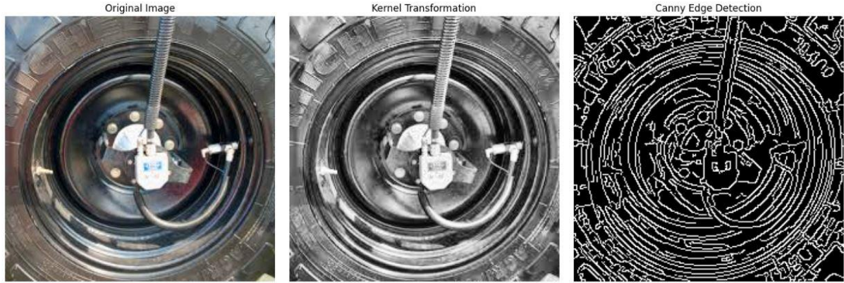
Figure 3.5 Canny Edge Detection on the low quality image after Kernel Transformation
