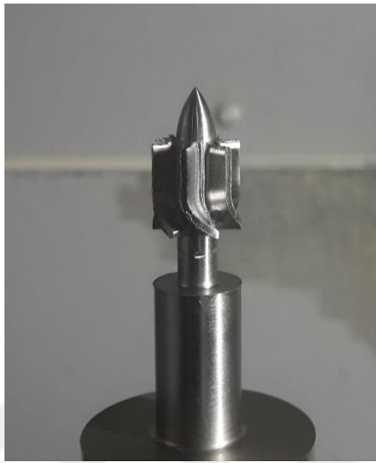
Figure 6.6: Diffuser of prototype II after machining
