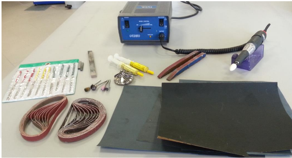
Figure 6.7: Polishing equipment containing sandpaper, diamond polish and rotary head [96]
