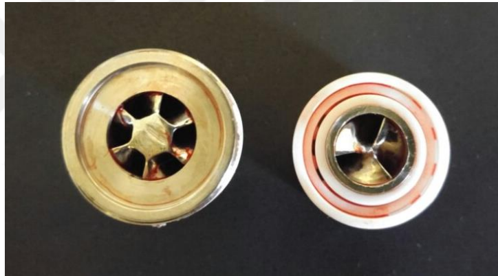
Figure 6.16: Disassembled pump after blood test diffuser (left) and impeller (right)
