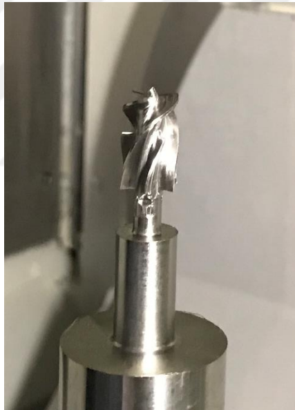
Figure 6.5: Impeller of prototype II after machining
