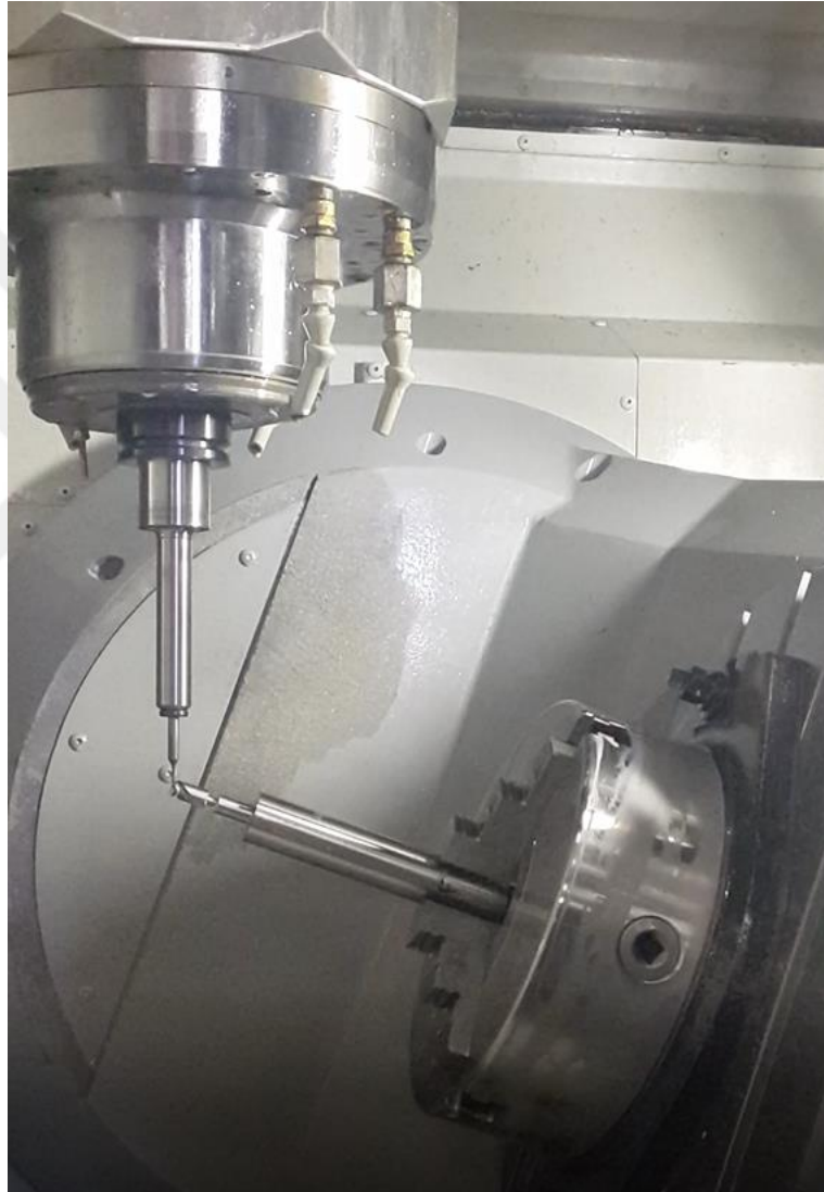
Figure 6.4: Impeller during the machining process
