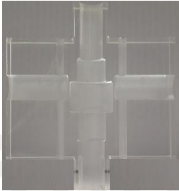
Figure 4.9: Machined plexiglass for single phase motor design
