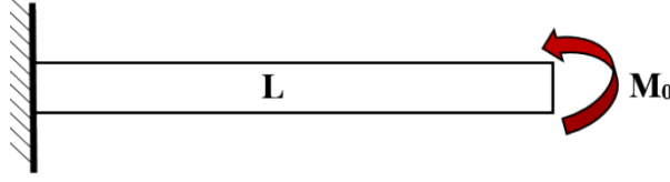
Figure 3.2: Moment acting to the free end of cantilever beam with small deflections.
