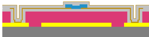
f) Deposition absorber layer with the second isolation layer.
