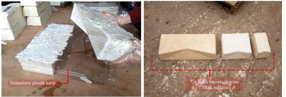
Şekil 37. Hy-Fi Tower statik kalıplama (Holcim Foundation for Sustainable Construction, 2014)
