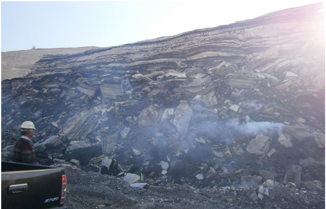
Figure 10. Self combustion at Hüsamlar Mine
