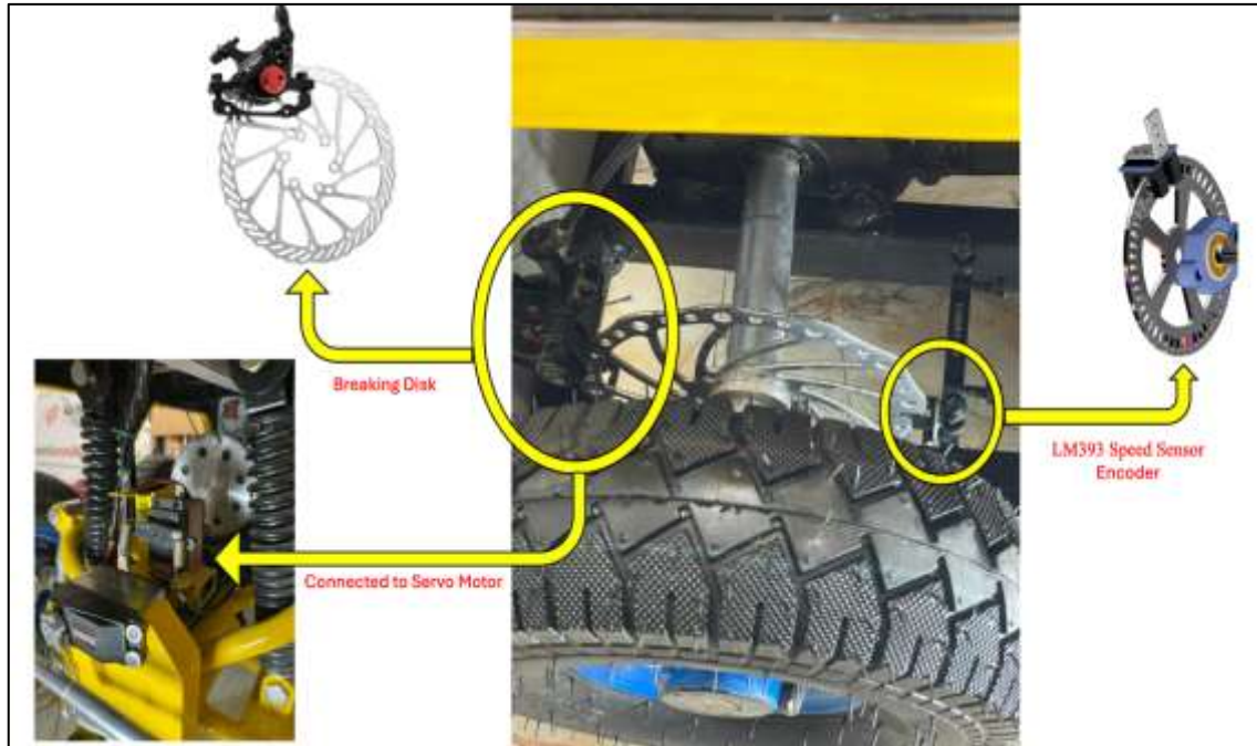
Figure 3.8: Braking and Encoding Systems.
