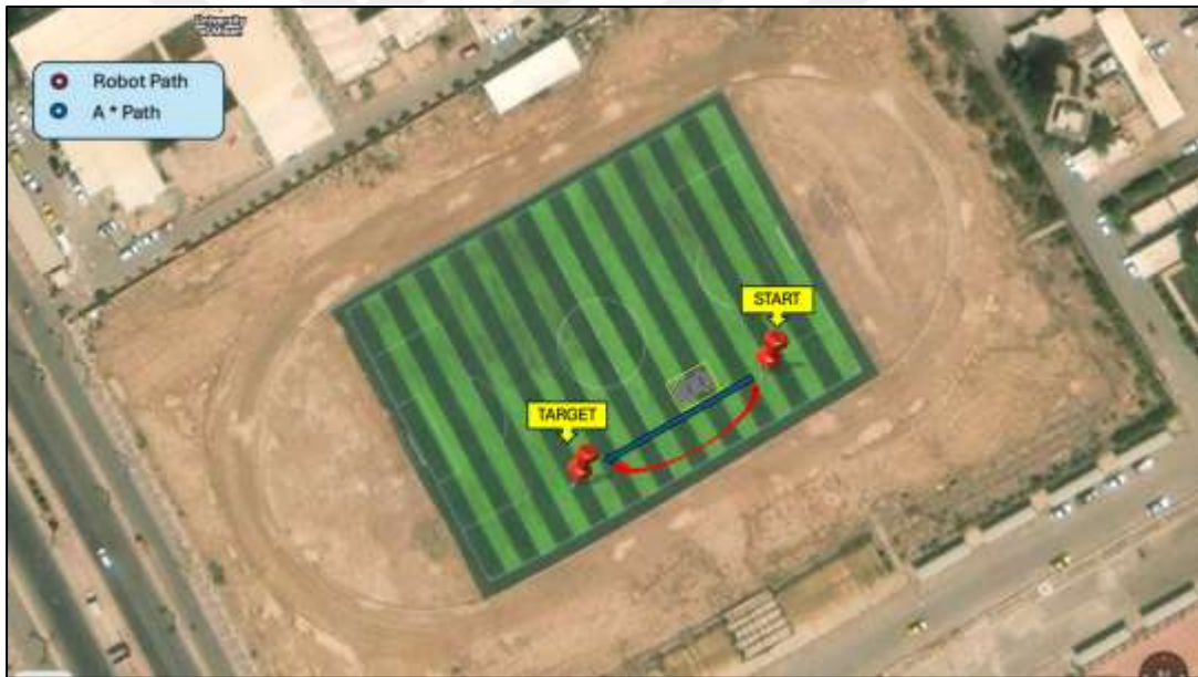
Figure 4.8: The Selected Path from A* Algorithm with Real Path from Vehicle.
