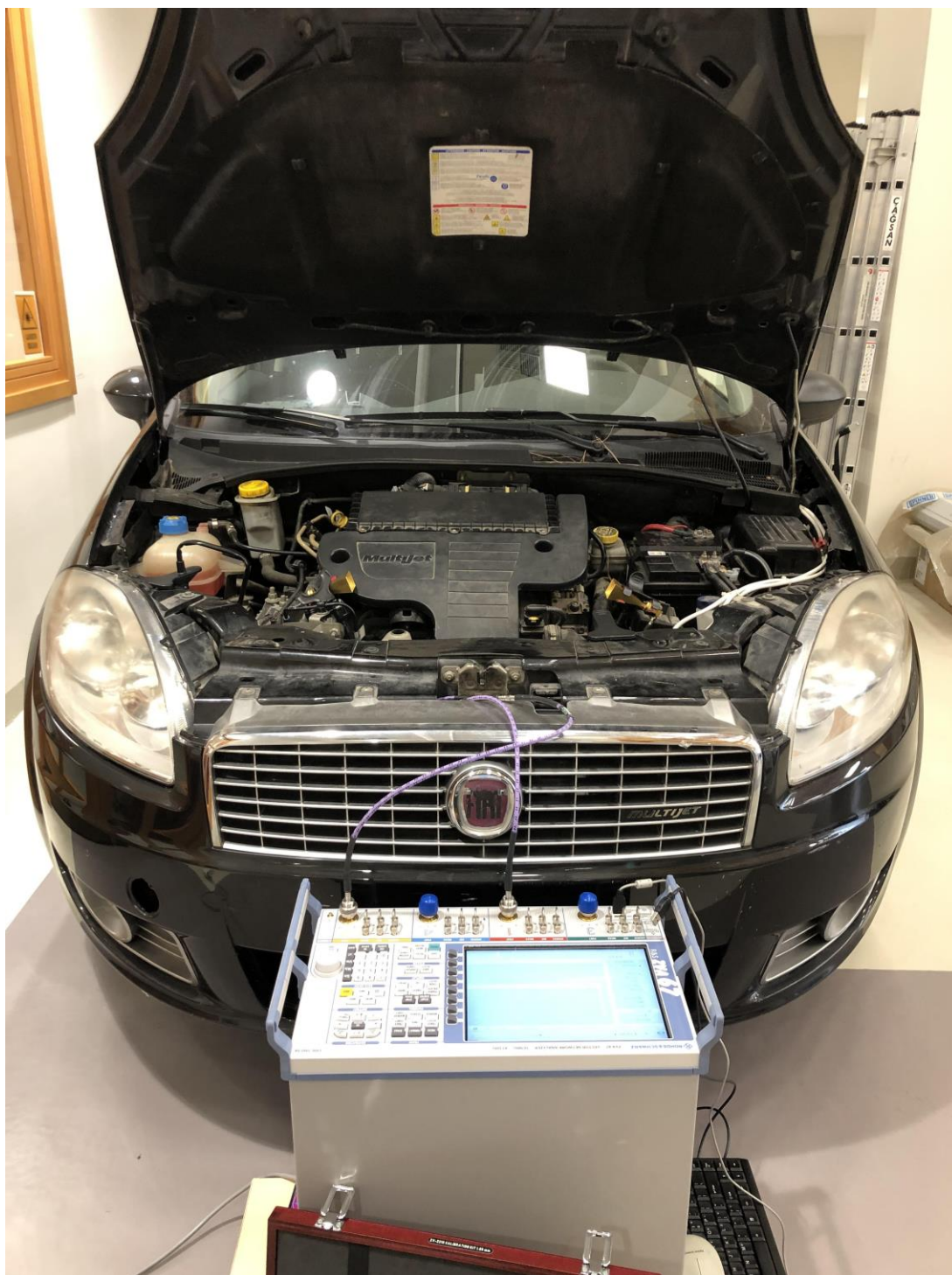
Figure 2.2: Sample measurement setup in Fiat Linea MY 2009.
