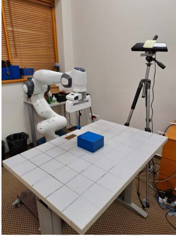
Figure 1.1: The real-robot setup. The robot holds a stick with a small ball at the end to interact with the objects. A RGBD camera is used for perception.
