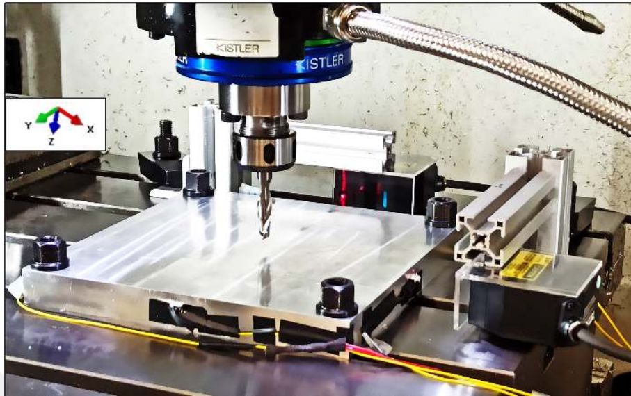
Figure 4.8: Workpiece clamping and installation of laser sensors.
