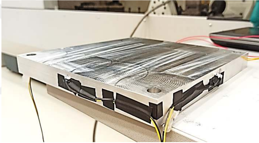
Figure 4.7: Thermocouple installation on the workpiece.
