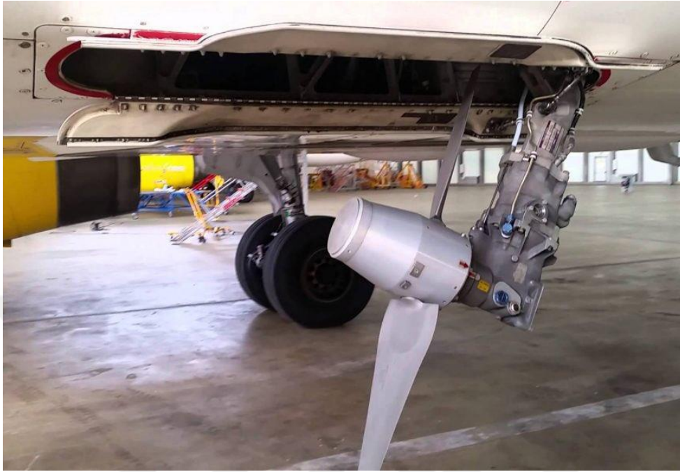
Figure 2.20. Located on a commercial aircraft The RAT mechanism was pulled out during maintenance on the ground (Mark Goertzen, 2016).
