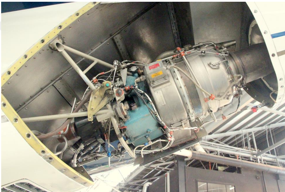
Figure 2.11. Position of a conventional Airbus A320 in the auxiliary power unit and tail section (Wikipedia, 2014).
