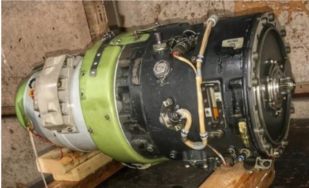
Figure 2.7. Integrated Drive Generator structure, the black part CSD, and the green part of the two are combined into a single block.
