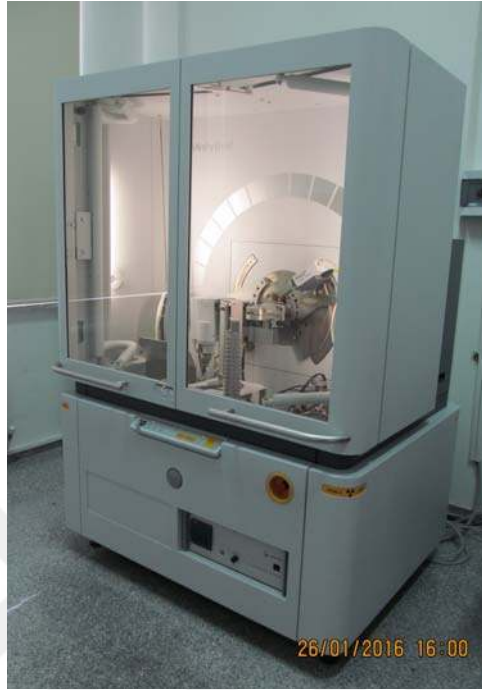
Figure 3.15. PANalytical Empyrean X-ray diffractometer used in the study
