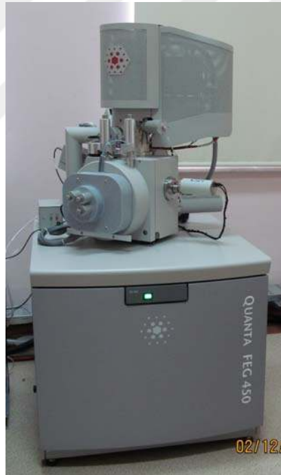
Figure 3.6. FEI Quanta FEG 450 including Field Emission Gun-Scanning Electron Microscope with Environmental Scanning Electron Microscope (ESEM) used for the imageVickers hardness specimens in this study
