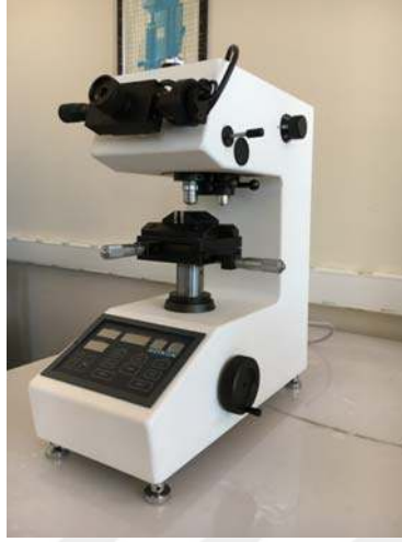
Figure 3.5. Metkon MH3 microhardness tester used in this study
