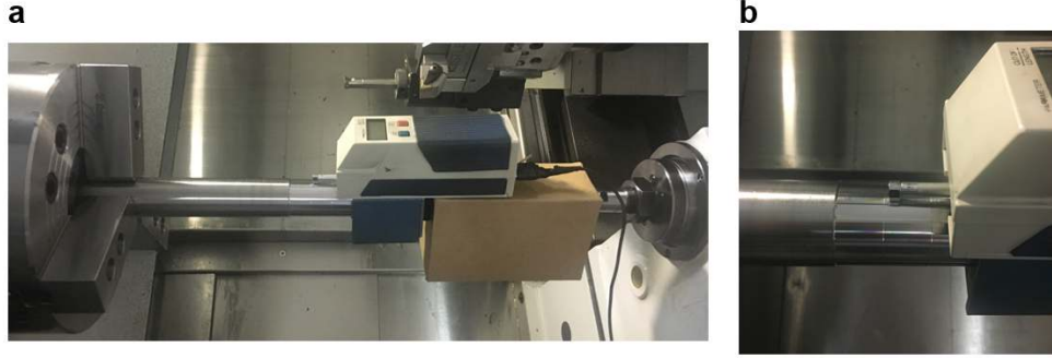
Figure 3.25. Mitutoyo SJ211 Surftest Surface Roughness Tester; a) Setup, b) Close-up shot.
