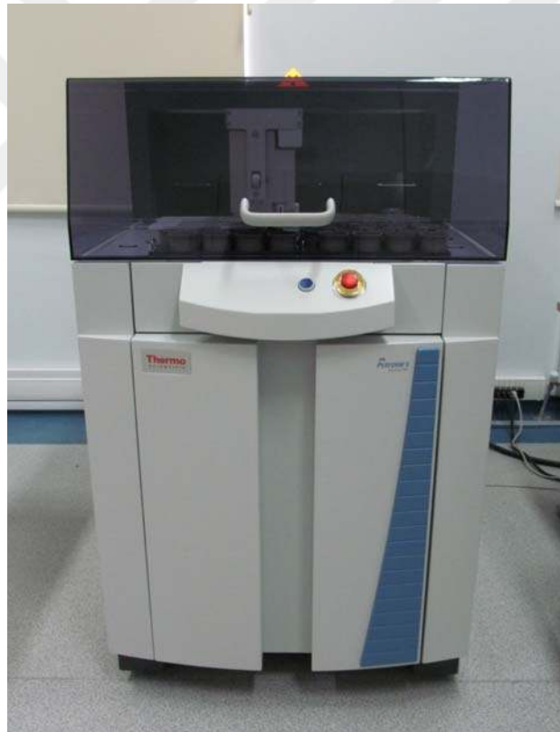
Figure 3.2. Thermo Scientific ARL PERFORM'X XRF Sequential X-Ray Fluorescence Spectrometer used for material analysis in this study
