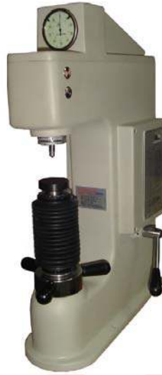
Figure 3.11. BMS 200-RB Analog Rockwell & Brinell Hardness Tester used in this study
