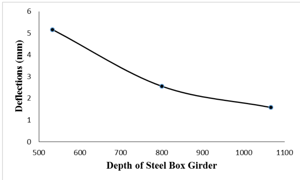
b) Deflection Vs. Box girder depth
