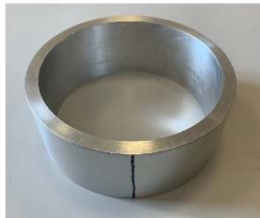
3) Aluminum tube (inner \phi 138 mm - outer \phi 158 mm, thickness of 8 mm)
