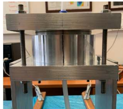
(8) Place the upper mold half on top of the upper perforated disk
