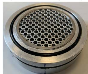
6) Upper perforated disk ( \phi 138mm), stainless steel glued to the upper flange (inner \phi 90 mm - outer \phi 98 mm)
