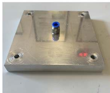
7) Aluminum upper mold half (outlet \phi 12 mm)
