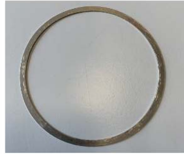
4) Stainless steel lower flange (inner \phi 90 mm - outer \phi 98 mm, thickness of 0.5 mm)
