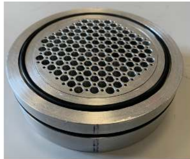
2) Lower perforated disk ( \phi 138 mm)
