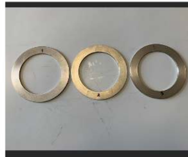
5) 3 metal rings each for different V_f , ( t = 3.53\text{mm}, 3.76\text{mm}, 4.22\text{mm} ), (inner \phi 100mm mm - outer \phi 138 mm)
