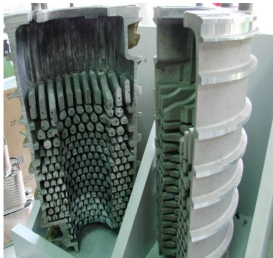
Figure 2.8 Cross-sectional view of one of the reference heat cell (HC).
