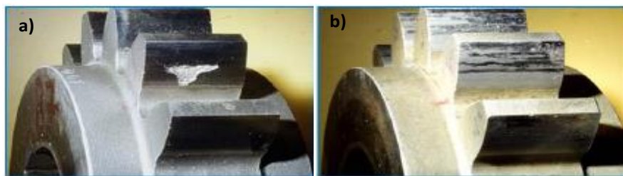
Figure 2.2 Common Gear Failure Modes in Aviation: a) Pitting; b) Micro Pitting (Tobie et al., 2017).
