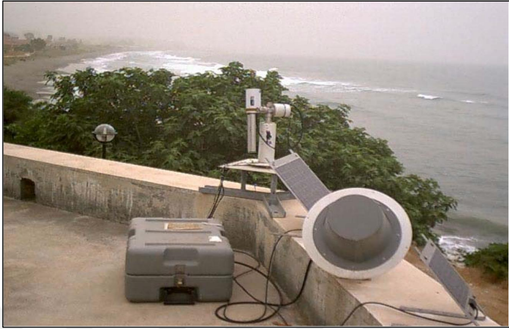
Figure 2.1 Sun photometer used at AERONET station in Erdemli district of Mersin (Kubilay & Koçak, 2009)
