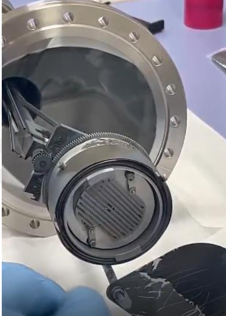
Figure 3.4: a picture of the bottom of the growth stage showing the heater coil and the rotation gears.
