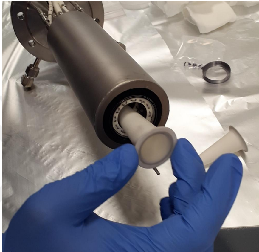
Figure 3.2: a picture of one of the effusion cells used in our MBE system.
