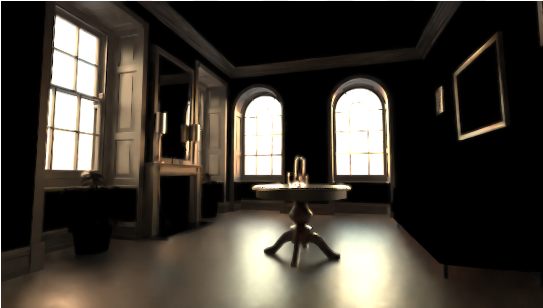
Figure 3.18: Denoised and guided upsampled specular component of the example scene rendered at R_{LR} , 640x360, with SPP_{OUR} , 32 SPP, upsampled to R_{HR} , 1280x720.
