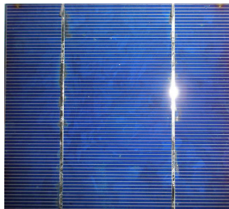
Figure 5.1.1.2 Unpackaged silicon monocrystalline solar cell
