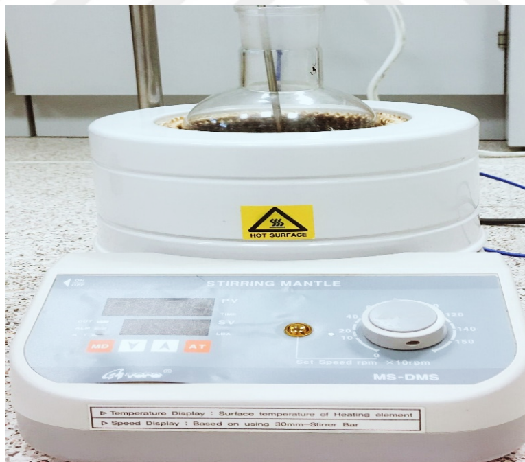
Figure 3.1: MS-DMS Stirring Heating Mantles applied during oxidation of SN 150 base oil
