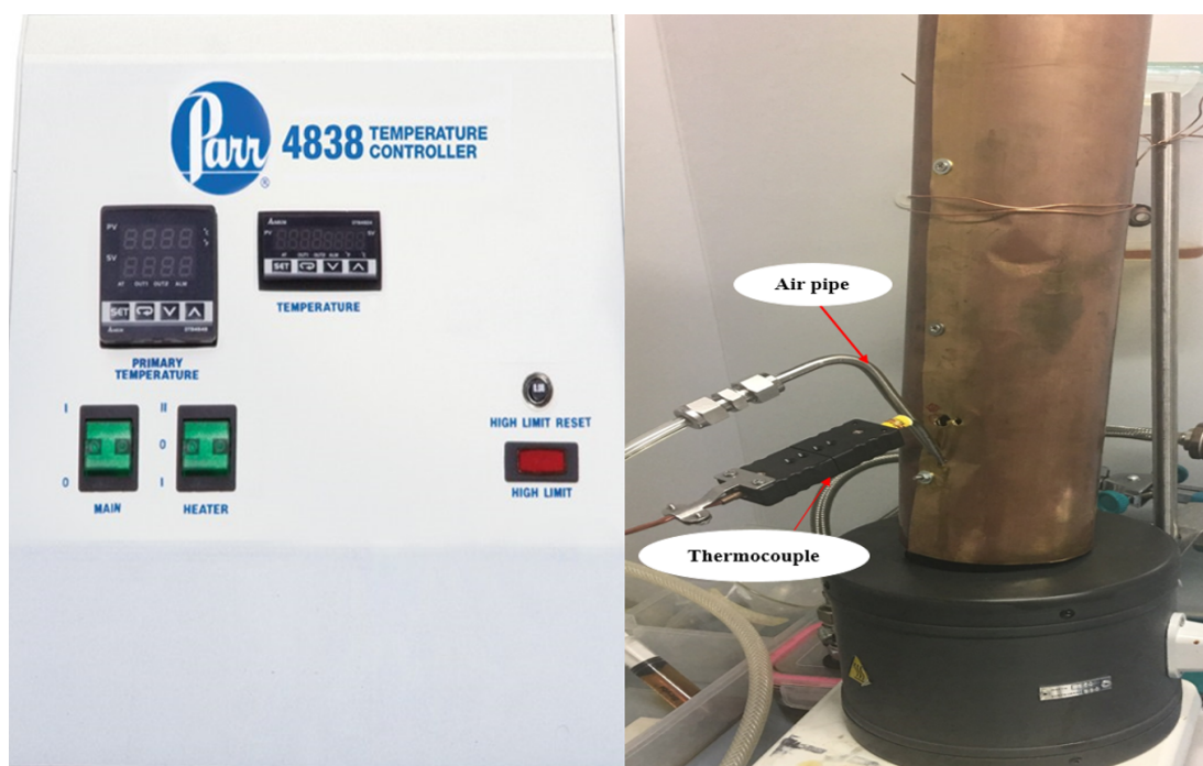
Figure 3.4: Reactor (left) and reactor control panel (right)
