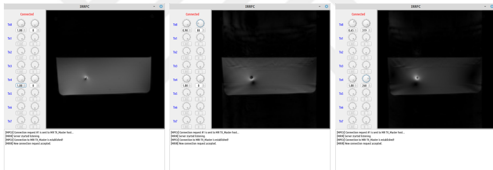
(a) Image at initial time point: no GRAPPA artifact (b) Channel eight phase modified: visible GRAPPA artifacts (c) Reverse polarization towards lateral sides: visible GRAPPA artifacts
