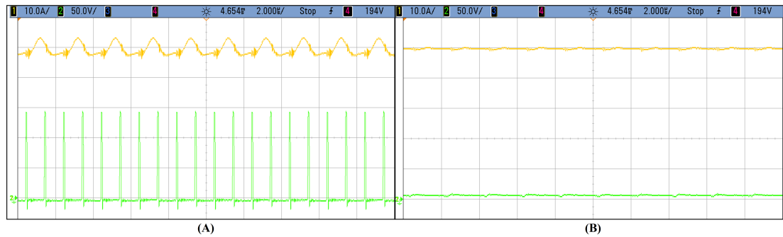
Figure B.5: Zoomed current (top) and voltage (bottom) applied to the coil without (A) and with (B) filter. Peak-to-peak ripple current is reduced more than twelve times by using the LC filter. Small resistance of the coil (about 200\text{m}\Omega ) requires small voltage levels and PWM duty cycle.
