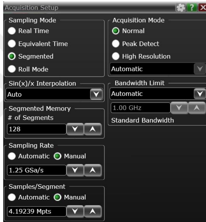
Fig 3.14 – The 'Acquisition Setup' settings implemented for the 'Segmented Sampling Mode' of the oscilloscope, used to record the consecutive gate and output waveforms of the amplifier
