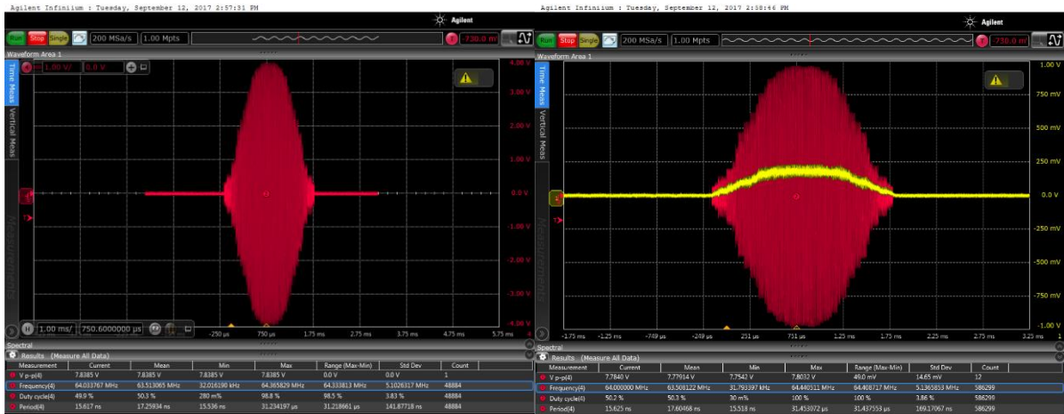
Fig. 4.18 – Gate modulated output waveform (red) of the amplifier when the carrier bit-stream designed for a duration of 2 ms is implemented. The overlapped drain current profile (yellow) is also shown (right side).
