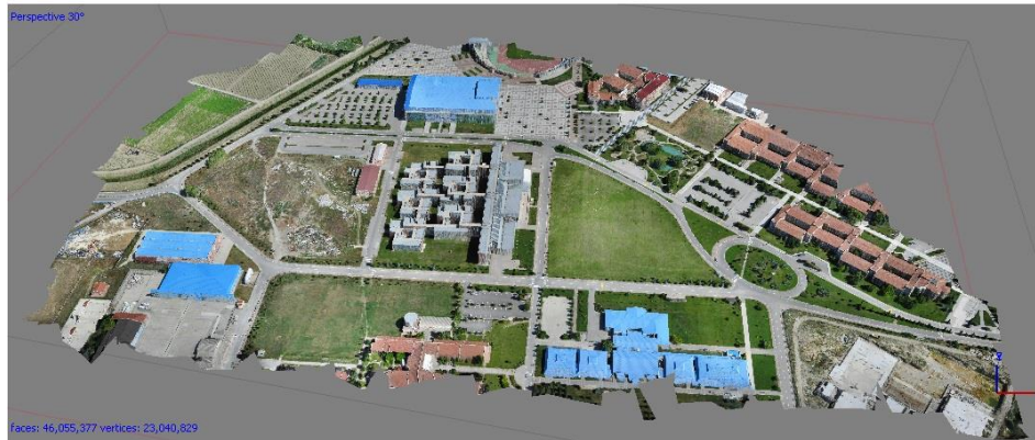
Figure 4.22. 3D view of the textured mesh model generated using PhotoScan.
