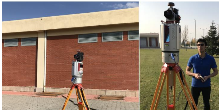
Figure 4.6. RIEGL VZ-2000 TLS during scanning
