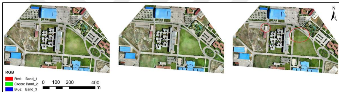
Figure 5.69. Comparison of orthomosaics generated using PhotoScan (left), Pix4D (middle), and 3Dsurvey (right).
