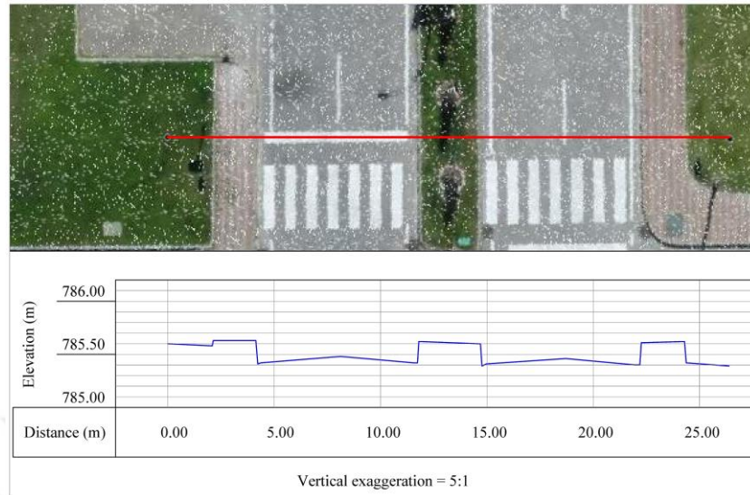
Figure 5.37. Cross-section of the road extracted from the TLS point cloud.
