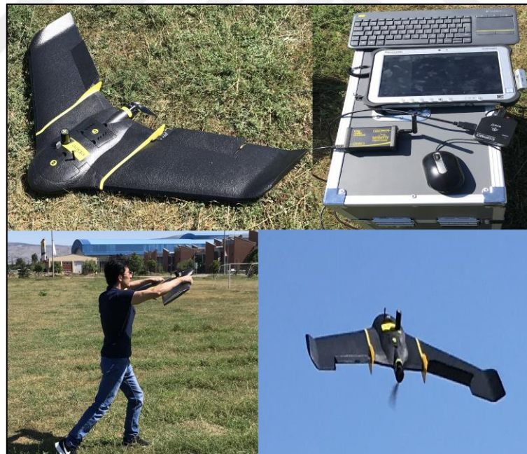
Figure 4.3. SenseFly eBee Plus with its ground control system during fieldwork
