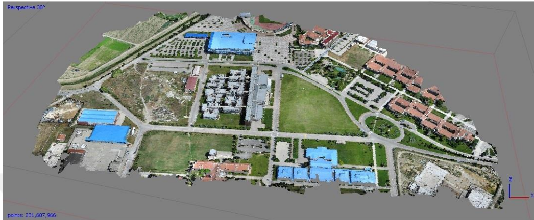
Figure 4.20. 3D view of dense point cloud generated using PhotoScan.
