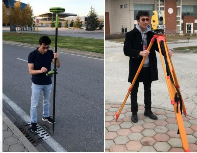
Figure 4.9. RTK DGNSS and TS measurements of ground control points.
