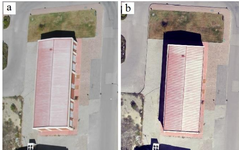
Figure 3.16. (a) raw aerial image and (b) rectified orthoimage.
