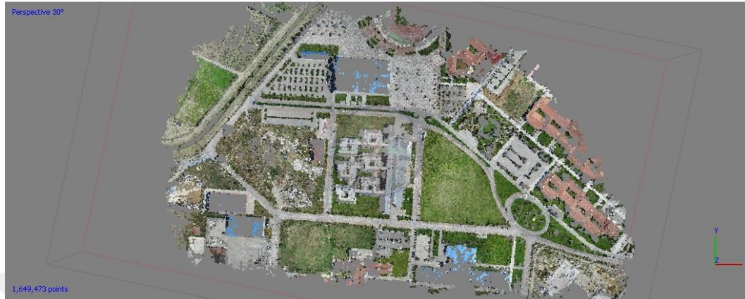
Figure 4.19. Sparse point cloud generated using PhotoScan.
