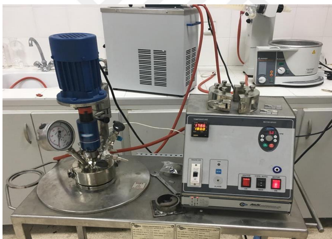
Figure 3.1. Hydrothermal set-up for synthesis of BFO and Yb-doped BFO.
