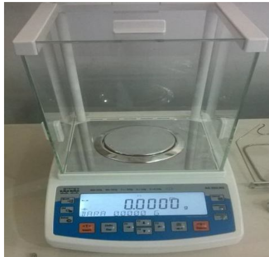
Şekil 2.14. Radwag AS 220 /C/2 hassas terazi
