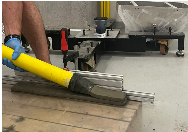
Figure 3.4: 3D-printing of cement-based mortars
