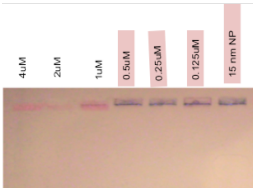
Figure 3.51 : Agarose gel result of DsRed-Au NP conjugate after addition of 1.5 M of NaCl salt solution.
