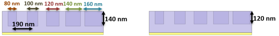
Figure 5.17: Nano-optical absorbers involving holes with higher depths
