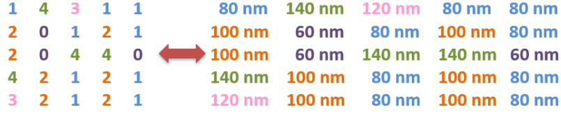
Figure 5.35: Optimal matrix representation and the corresponding depth values for higher maximum power density enhancement at 535 THz
