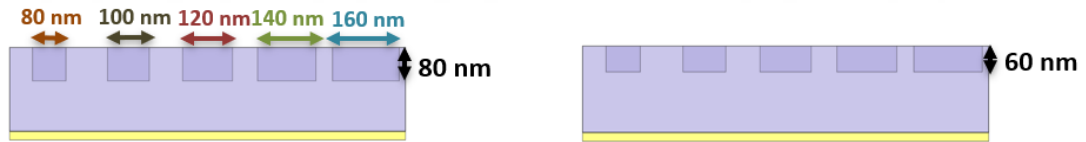
Figure 5.21: Nano-optical absorbers involving holes with lower depths
