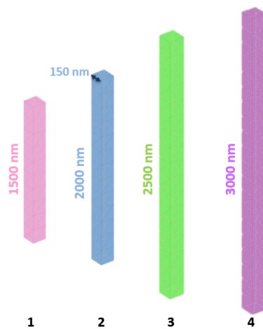
Figure 3.5: Dielectric rods used in optimization of rod lengths
