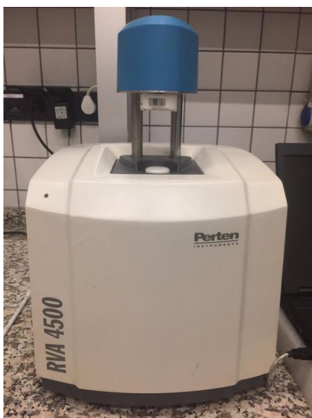
Figure 3.10. Rotational viscometer with variable temperature and shear capabilities
