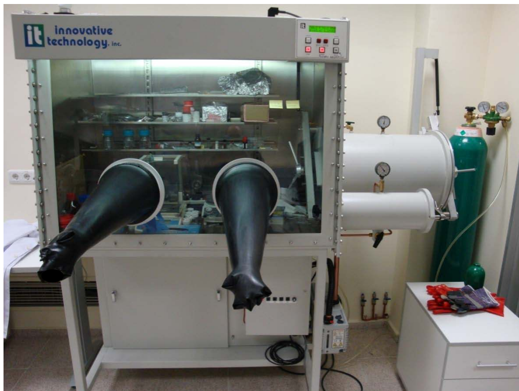
Figure 2.1.3 Glove box (nitrogen filled), used for storage and preparation of the chemicals used in the synthesis at the Demir Lab.
