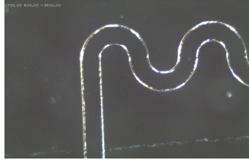
Figure 4.4: Microscope image of sinusoidal section of conjugated polymer microreactor
