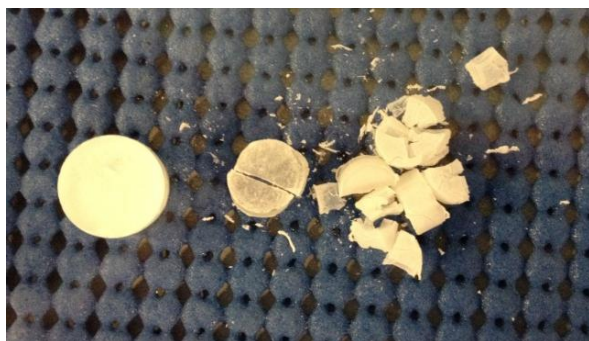
Figure 4.16: Comparison of 3 drying methods: (from left to right) Supercritical drying, oven drying at 50°C, ambient pressure drying
