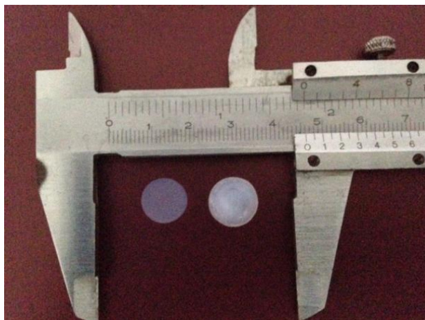
Figure 4.5: Photos of a silica aerogel (left) and a silica aerogel encapsulated with an alginate aerogel layer (right)
