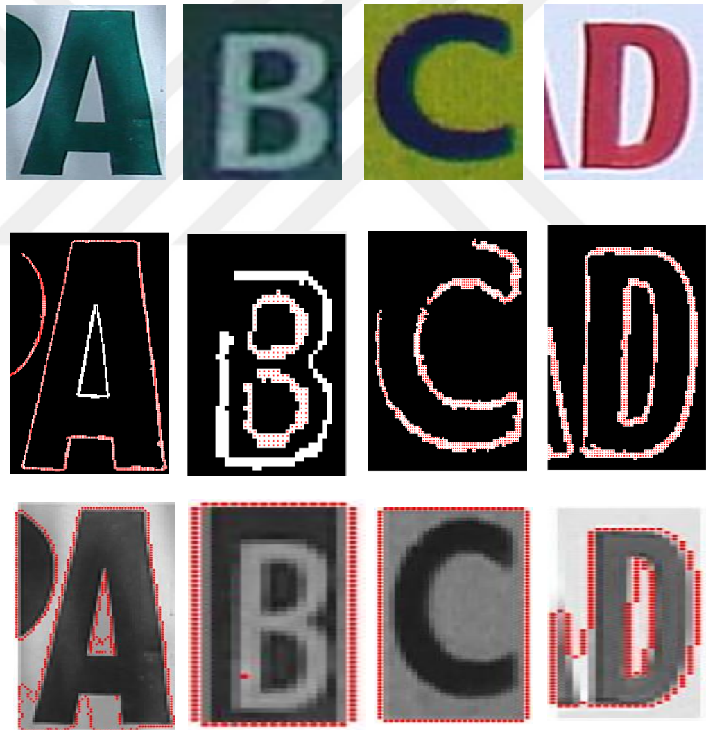
Figure 6.3. Keypoint detection: original images (first row), designed method (second row) and SIFT
