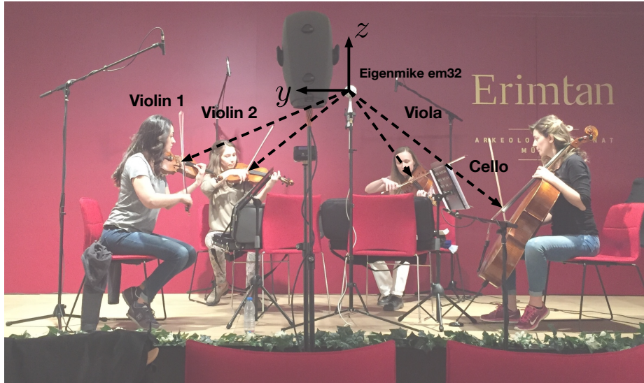
Figure 4.9: Setup for the recording of the classical quartet. Position of the microphone array and directions of the instruments are indicated.©2018 IEEE [1]
