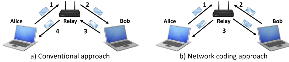
Figure 1.3: Conventional (a) vs. network coding (b) approach. 3 transmissions instead of 4 saves 1 transmission cycle for any other data exchange.
